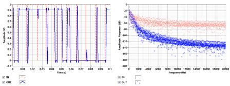
Fig. 5: Comparison of input and output of FIR low-pass filter for triangular, also known as Bartlett, window. a) time domain, b) frequency domain.
