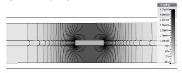
Fig. 3: The employed suspended stripline cross-section with electrical field distribution computed by the CST Studio
