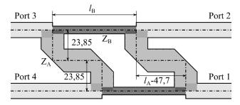
Fig. 9: The vertical feeder dividers layout
