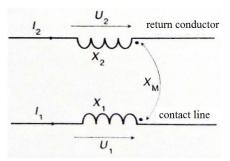
Fig. 5 The scheme of the booster transformers [7]
