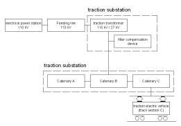
Fig. 1: Traction circuit of power supply system of AC 25 kV
