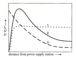
Fig. 7 The voltage run on rails in dependence on the distance from power supply station  $(1 \dots [U^c]$ - when the traction current is constant;  $2 \dots [U]$  - when there is a short-circuit;  $3 \dots [IK]$  - process of short-circuit current  $)^{[3,4]}$
