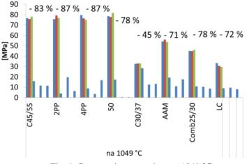
Fig. 4: Compressive strength, max 1049 °C
