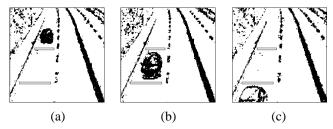
Fig. 6. Images after conversion into the binary form and smoothing operations with the marked detection fields: a) i = 10, b) i = 34, c) i = 49
