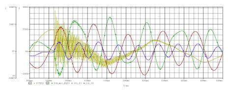
Fig. 3: The voltage and current waveform at FCD
