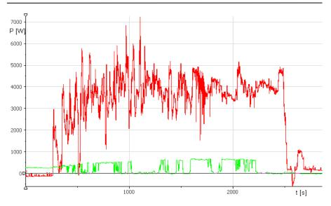
Fig. 3: Traction power (RED) and power of photovoltaic generator (GREEN) during one of the first testing drives
