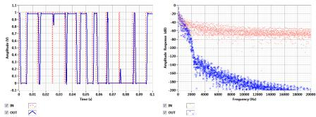
Fig. 8: Comparison of input and output of FIR low-pass filter for Blackman window. a) time domain, b) frequency domain.
