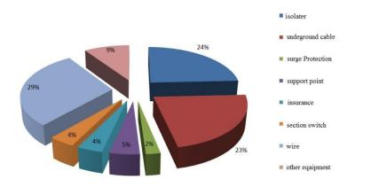
Fig. 8: The distribution of the effect of selected damaged elements at SAIFI for MV (all categories) from 2008 to 2013 [authors]
