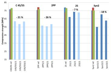
Fig. 13: Compressive strength after loaded by local fire
