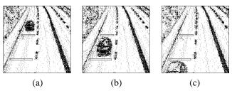
Fig. 5. Images after conversion into the binary form with the marked detection fields: a) i = 10, b) i = 34, c) i = 49
