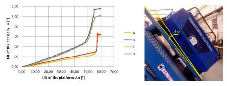
A – blocked suspension, B – blocked upper suspension, C – blocked lower suspension, D – unblocked suspension
