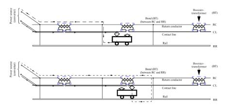
Fig. 4 The return current way on AC system with the boostertransformers<sup>[7]</sup>
