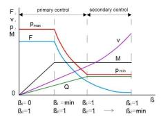
Fig. 4: Control characteristic of HS transmission
