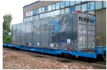
Fig. 3: TelliBox on low Sffggmrrss type train [6]
