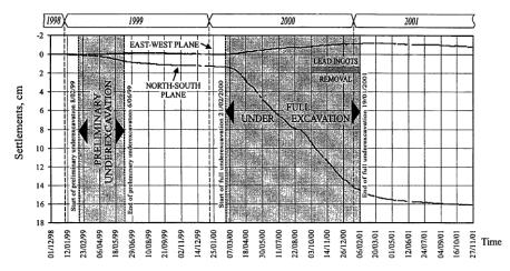
Fig. 3: Time-Settlement Diagram of the Leaning Tower of Pisa [2]
