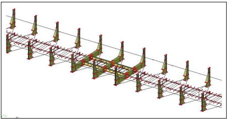
Fig. 3: Combination of beam – 1D and plate elements – 2D (ESA PT)
