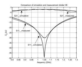
Fig. 6: The measured vs simulated S parameters of the divider H5 comparison
