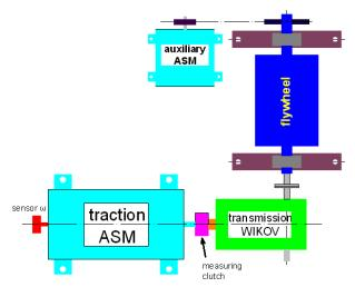
Fig. 1. The conception of the laboratory test stand
