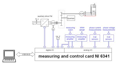
Fig. 2. The electrical structure of the laboratory test stand
