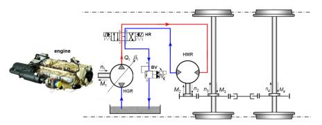
Fig. 3: Scheme of one hydraulic circuit
