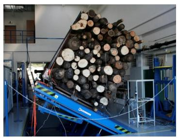
Fig. 1: Experimental determination of force distribution along the stanchion
