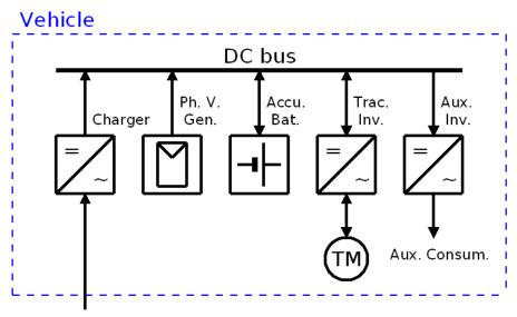
El. Net Fig. 2: Block diagram of traction power circuit
