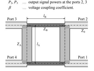
Fig. 5: One stage branch line divider circuit diagram
