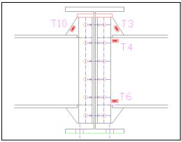
Fig. 12: Strain gauge positions
