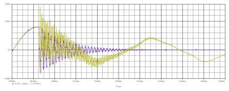
Fig. 2: The voltage waveform at FCD and recuperation mode of vehicle
