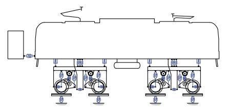
Fig. 1: Multi-body mechanical model of an electric locomotive for purposes of drive dynamics simulations
