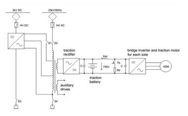
Fig. 1: Two power supplies railway vehicle
