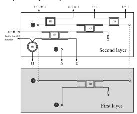
Fig. 7: The double layer structure of the horizontal feeder central section
