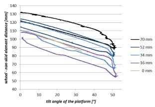
Fig. 5: Dependence between lateral movement of the wheel and height of non-skid member during tilting of the platform
