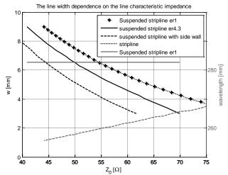
Fig. 4: The line width and wavelength dependence on the line characteristic impedance for the suspended stripline and substitutive configurations.
