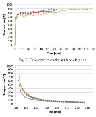
Fig. 3: Temperature on the surface - cooling
