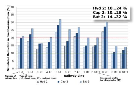
Fig. 3: Simulation results for "heavy" hybrid configurations
