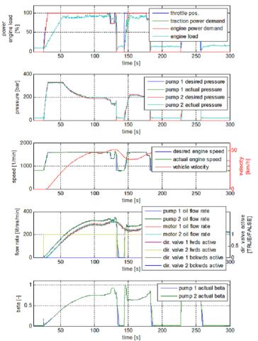
Fig. 9: Vehicle acceleration at 100 % throttle
