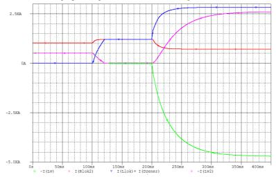
Fig.4: The theoretical current waveform flowing back to the traction substation
