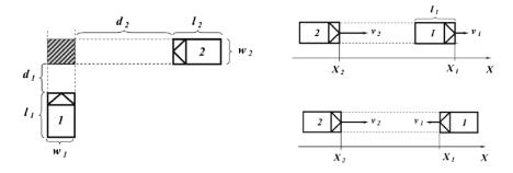
Fig. 2: TTC definition for three possible collisions (crossing, rear-end, lane change)
