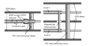
Fig. 10: The 50  $\Omega$  termination and the perpendicular interconnection design
