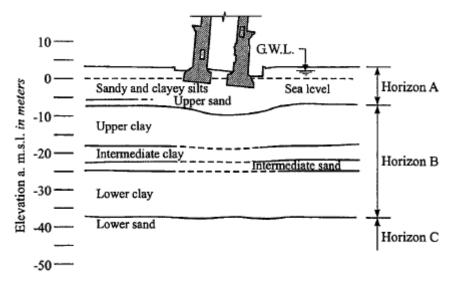
Fig. 1: Subsoil Profile of the Leaning Tower of Pisa [2]
