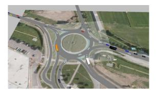
Fig. 6: Roundabout with spiral arrangement of lanes in PTV VISSIM
