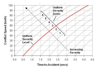
Fig. 4: Uniform severity level and severity zones developer by Hydén
