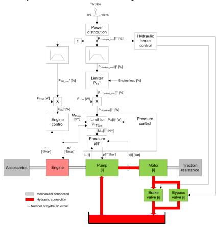
Fig. 7: Control structure
