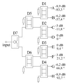
Fig. 8: The SSR antenna vertical feeder circuit diagram
