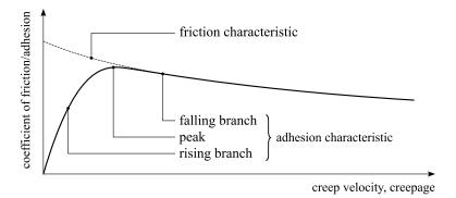
Fig. 3: Sketch of a basic adhesion characteristic together with a velocity-dependent function of friction
