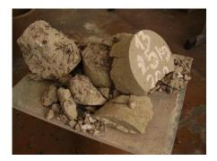
Fig. 8: Cylinder "25" (max. 1049 °C)
