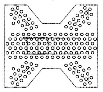
Fig. 7: Top View of Incheon Tower Foundations [7]
