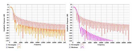
Fig. 3: Comparison of FIR low-pass filters for a) rectangular and Hamming and b) rectangular and Blackman windows.
