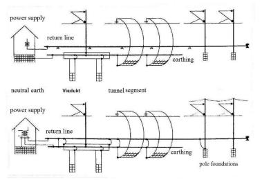
Fig. 1 The diagram of the earthing on electric rails (up.....DC system, down...AC system) [3, 4]
