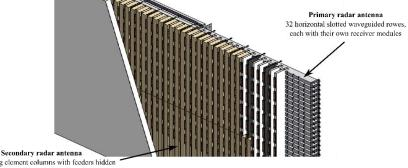
27 radiating element columns with feeders hidden in the polarization diaphragms of primary radar antenna
