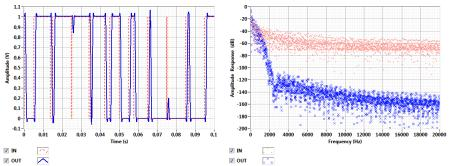
Fig. 6: Comparison of input and output of FIR low-pass filter for Hanning window. a) time domain, b) frequency domain.
