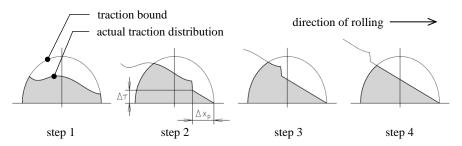
Fig. 5: Illustration to the simplified model of transient rolling – distribution of tangential stress in contact in transition from general initial state to steady rolling with constant creepage
