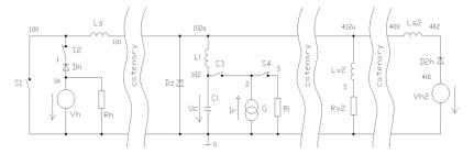
Fig. 2: The equivalent circuit for simulation of faults at recuperation
