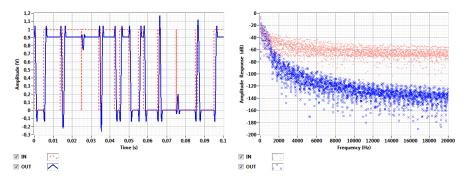
Fig. 4: Comparison of input and output of FIR low-pass filter for rectangular window. a) time domain, b) frequency domain.
