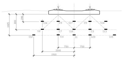
Fig. 1: Detailed description of pressure indicators placement
