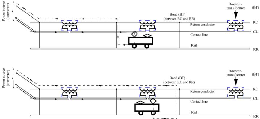
Fig. 4 The return current way on AC system with the boostertransformers<sup>[7]</sup>
