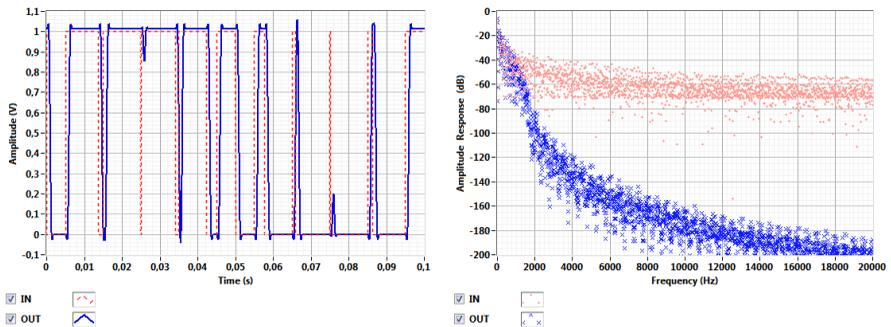
Fig. 7: Comparison of input and output of FIR low-pass filter for Hamming window. a) time domain, b) frequency domain.
