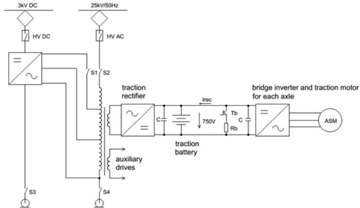
Fig. 1: Two power supplies railway vehicle
