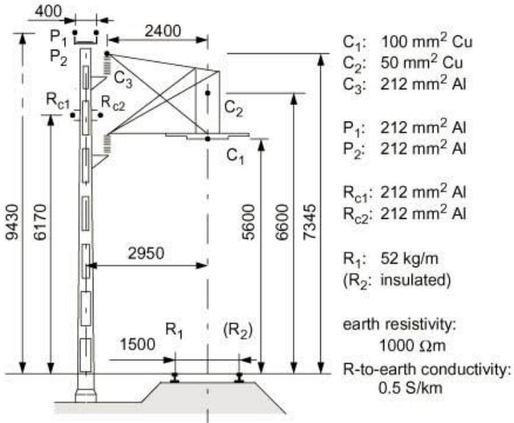
Fig. 6 The return conductors – the line configuration [3]
