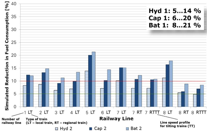
Fig. 2: Simulation results for "light" hybrid configurations
