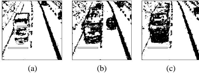
Fig. 13. Examples of images after conversion into the binary form of the two-layer image model including vehicles of various types: (a) a truck, (b) a bus, (c) an articulated lorry
