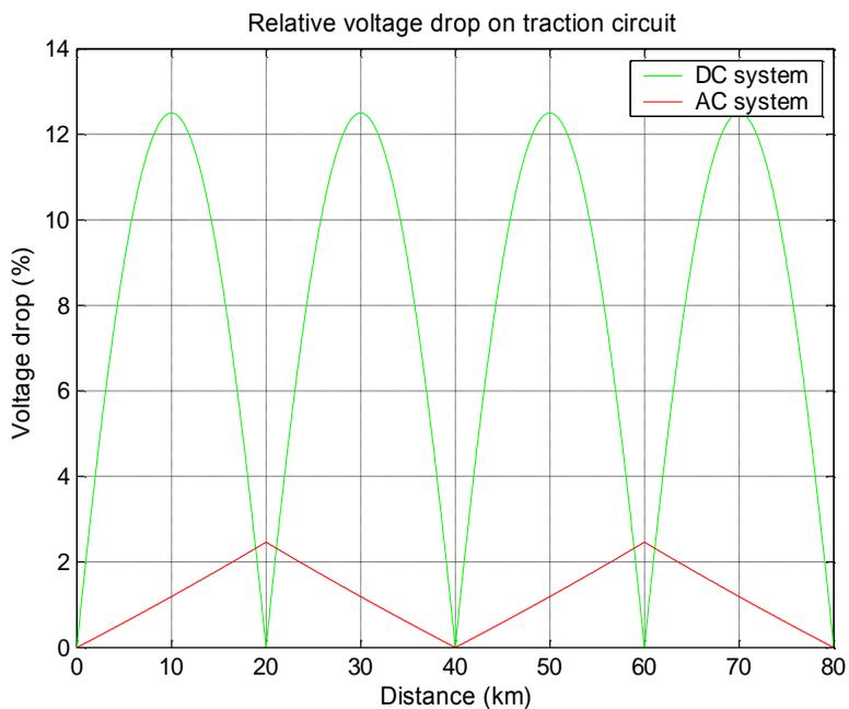
Attachment 3: Comparison of DC/AC systems – Power losses
