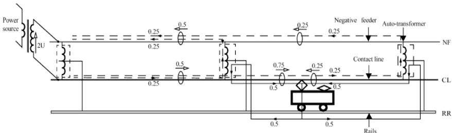
Fig. 3 The return current way on AC system with the auto transformers [7]
