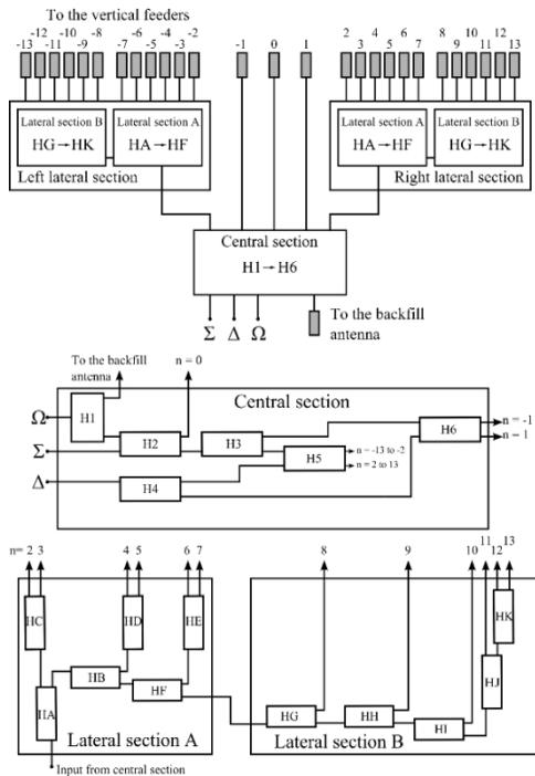
Fig. 2: The horizontal MSSR antenna feeder circuit diagram
