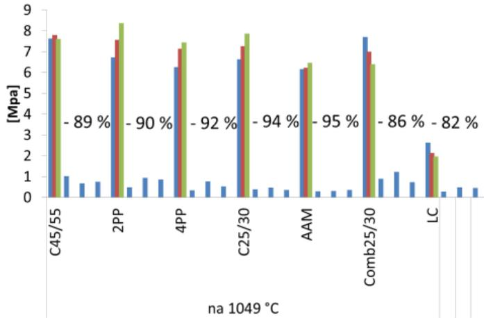
Fig. 5: Flexural strength, max 1049 °C
