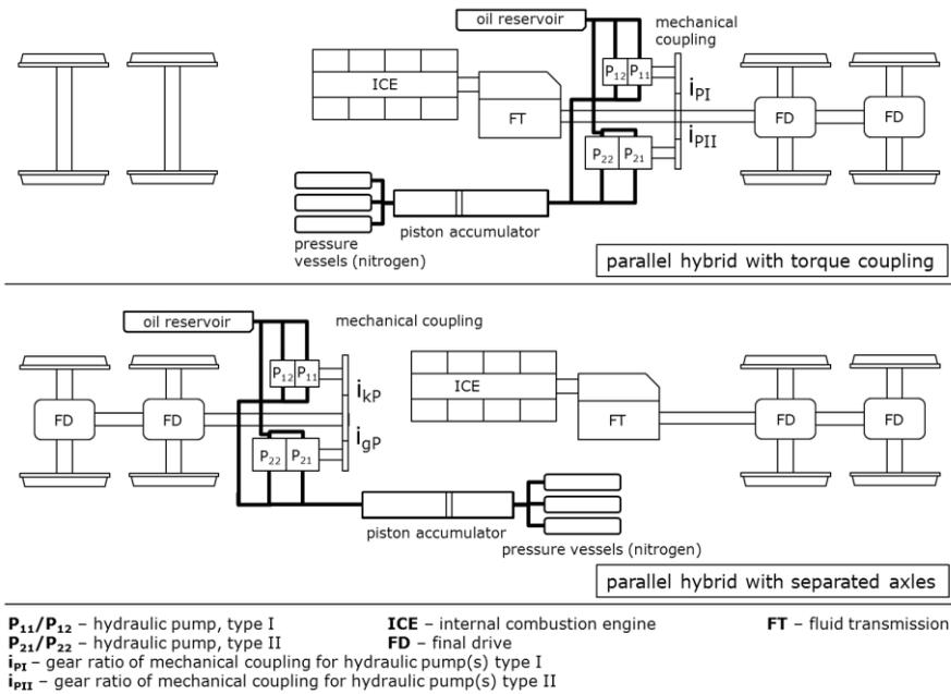
Fig. 1: Possible hydrostatic parallel-hybrid configurations
