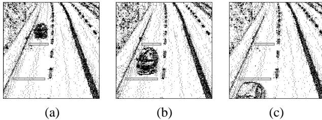
Fig. 5. Images after conversion into the binary form with the marked detection fields: a)  $i = 10$ , b)  $i = 34$ , c)  $i = 49$
