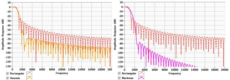
Fig. 3: Comparison of FIR low-pass filters for a) rectangular and Hamming and b) rectangular and Blackman windows.
