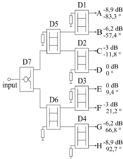
Fig. 8: The SSR antenna vertical feeder circuit diagram
