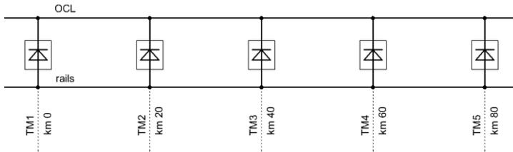
Fig. 4: Feeding diagram on DC system
