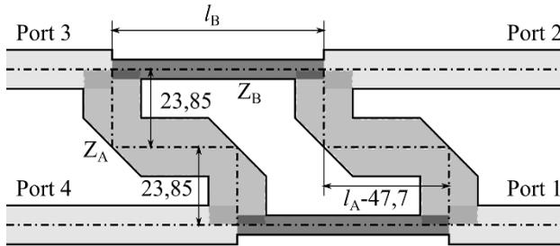
Fig. 9: The vertical feeder dividers layout
