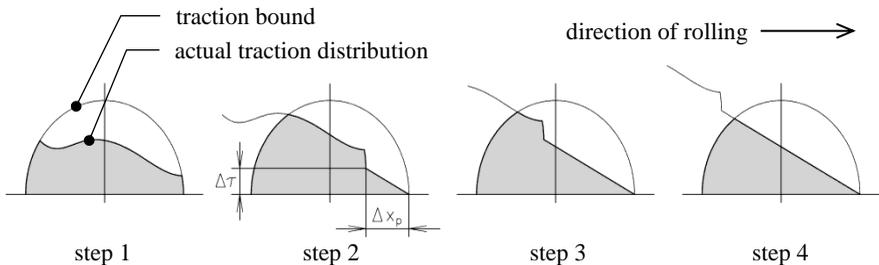
Fig. 5: Illustration to the simplified model of transient rolling – distribution of tangential stress in contact in transition from general initial state to steady rolling with constant creepage
