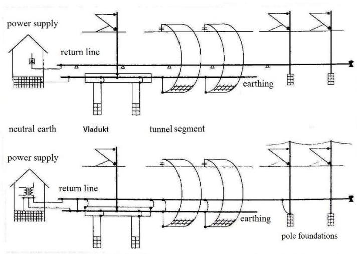
Fig. 1 The diagram of the earthing on electric rails (up.....DC system, down...AC system) [3, 4]
