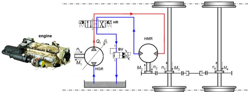
Fig. 3: Scheme of one hydraulic circuit
