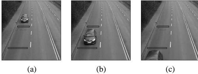
Fig. 3. Images from the input image sequence with the marked detection fields: a)  $i = 10$ , b)  $i = 34$ , c)  $i = 49$
