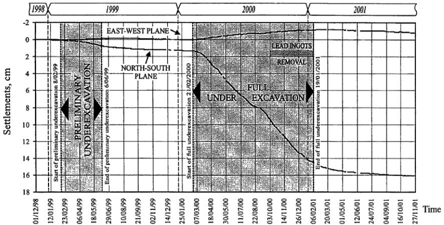
Fig. 3: Time-Settlement Diagram of the Leaning Tower of Pisa [2]
