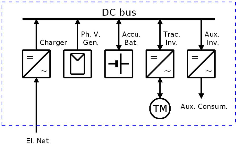
Fig. 2: Block diagram of traction power circuit
