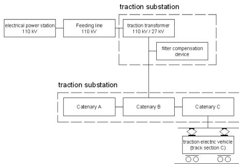
Fig. 1: Traction circuit of power supply system of AC 25 kV
