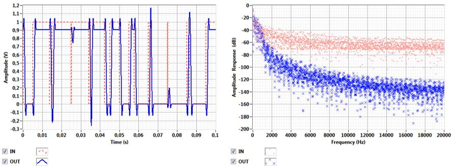
Fig. 4: Comparison of input and output of FIR low-pass filter for rectangular window. a) time domain, b) frequency domain.
