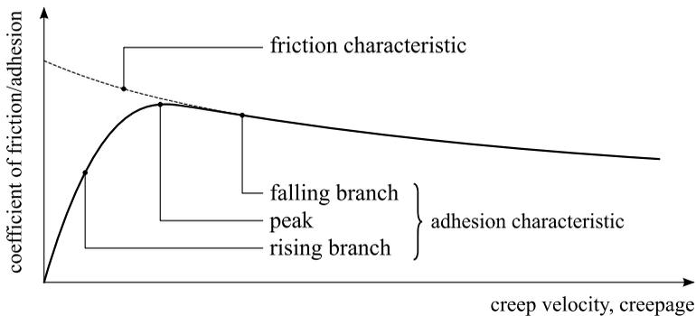
Fig. 3: Sketch of a basic adhesion characteristic together with a velocity-dependent function of friction
