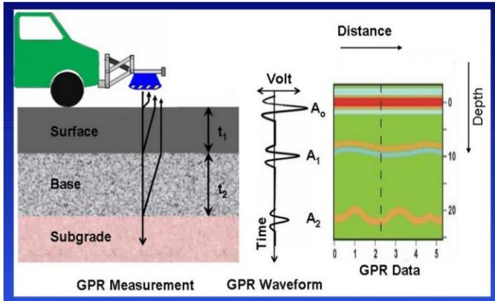
Fig. 1: GPR principle [2]
