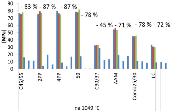
Fig. 4: Compressive strength, max 1049 °C
