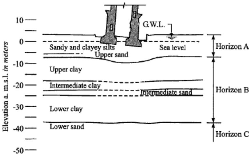
Fig. 1: Subsoil Profile of the Leaning Tower of Pisa [2]
