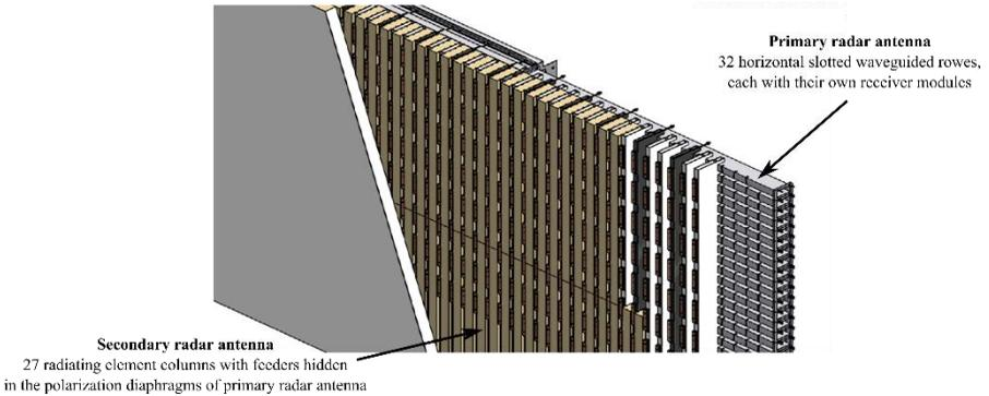
Fig. 1: The integrated PSR/SSR antenna design
