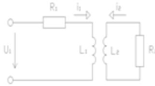
Fig. 5: The equivalent circuit for the theoretical derivation of the time response of the current to voltage jump  $U_1$
