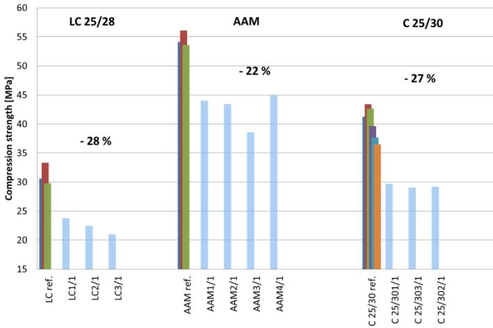
Fig. 12: Compressive strength after loaded by local fire
