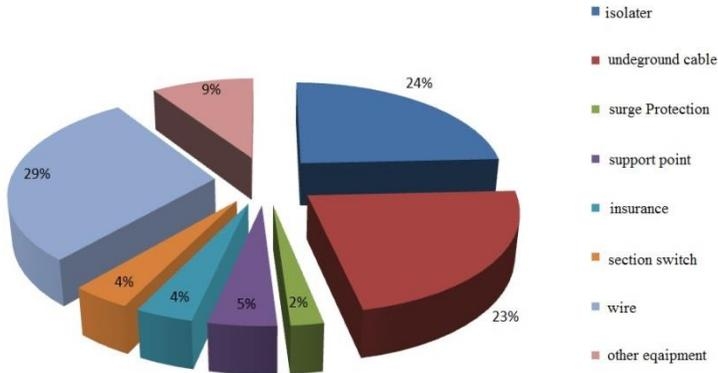
Fig. 8: The distribution of the effect of selected damaged elements at SAIFI for MV (all categories) from 2008 to 2013 [authors]
