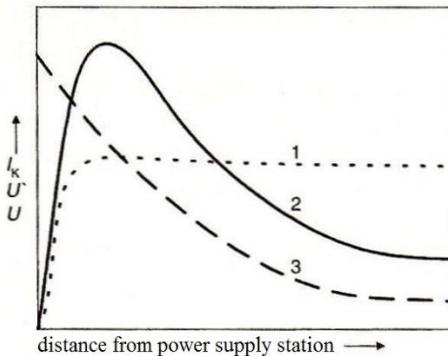
Fig. 7 The voltage run on rails in dependence on the distance from power supply station (1 ... [U']- when the traction current is constant; 2 ... [U] - when there is a short-circuit; 3 ... [I<sub>k</sub>] - process of short-circuit current) <sup>[3,4]</sup>
