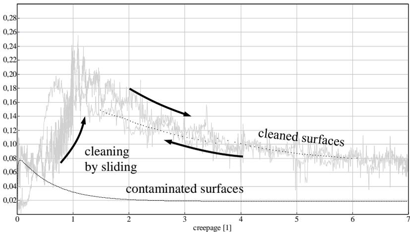
Fig. 4: One of transient adhesion characteristics measured at a roller rig (wheels contaminated with oil, rolling speed 10 km/h)
