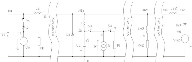
Fig. 2: The equivalent circuit for simulation of faults at recuperation
