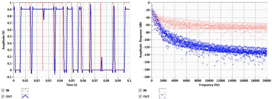
Fig. 5: Comparison of input and output of FIR low-pass filter for triangular, also known as Bartlett, window. a) time domain, b) frequency domain.
