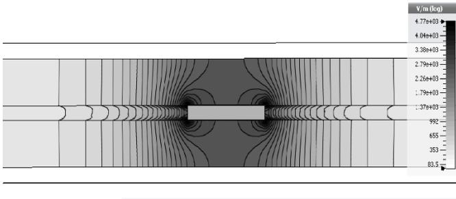
Fig. 3: The employed suspended stripline cross-section with electrical field distribution computed by the CST Studio
