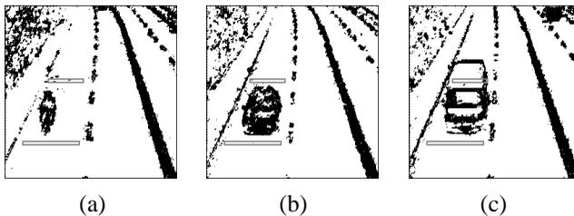
Fig. 11. Examples of images after conversion into the binary form of the two-layer image model including vehicles of various types: (a) a motorcycle, (b) a passenger car, (c) a minibus
