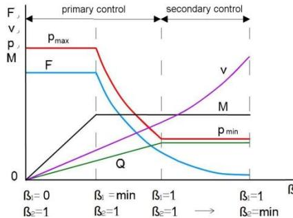
Fig. 4: Control characteristic of HS transmission
