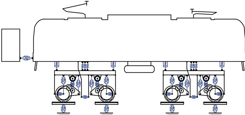
Fig. 1: Multi-body mechanical model of an electric locomotive for purposes of drive dynamics simulations
