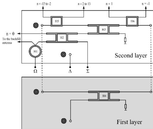
Fig. 7: The double layer structure of the horizontal feeder central section
