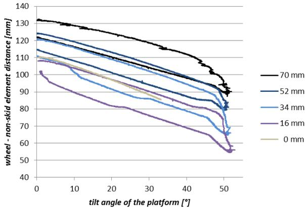
Fig. 5: Dependence between lateral movement of the wheel and height of non-skid member during tilting of the platform
