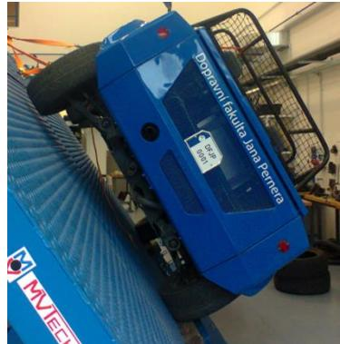
Fig. 3: Tilting platform in Teaching and Research Center in Transport
