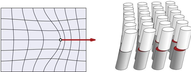
Fig. 2: Illustration to material models – left: continuum for exact theories of rolling contact; right: bristle model for simplified theories
