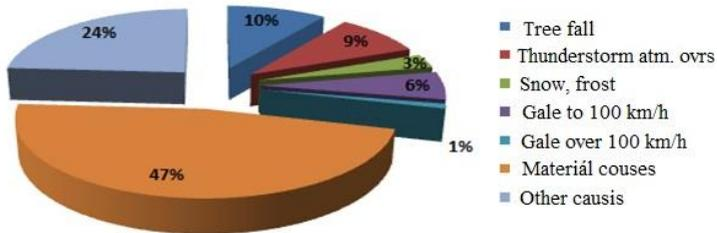
Fig. 7: The distribution of the number of unplanned events at lines according to the cause of origin [authors]
