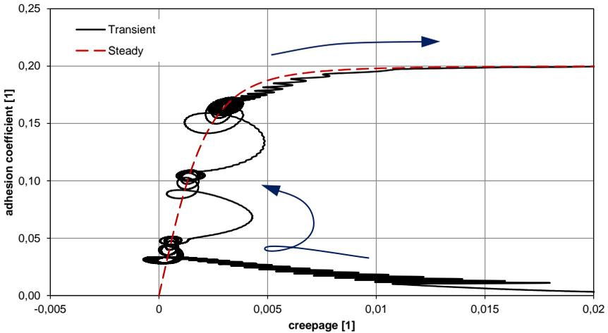
Fig. 6: Adhesion characteristic recorded in simulation of an accelerating locomotive using the simplified model of transient rolling
