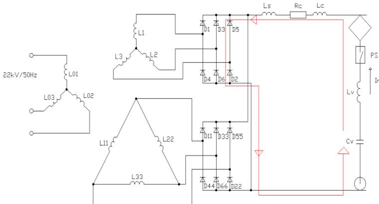
Fig. 1: The flow direction of recuperative current coming through the fault rectifier
