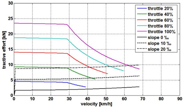
Fig. 6: Partial tractive effort curves of M27 after reconstruction
