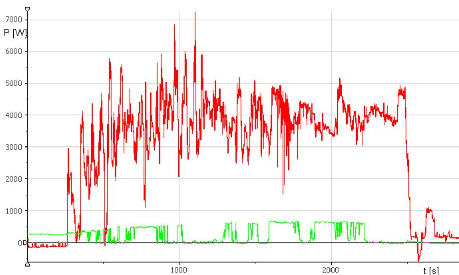
Fig. 3: Traction power (RED) and power of photovoltaic generator (GREEN) during one of the first testing drives
