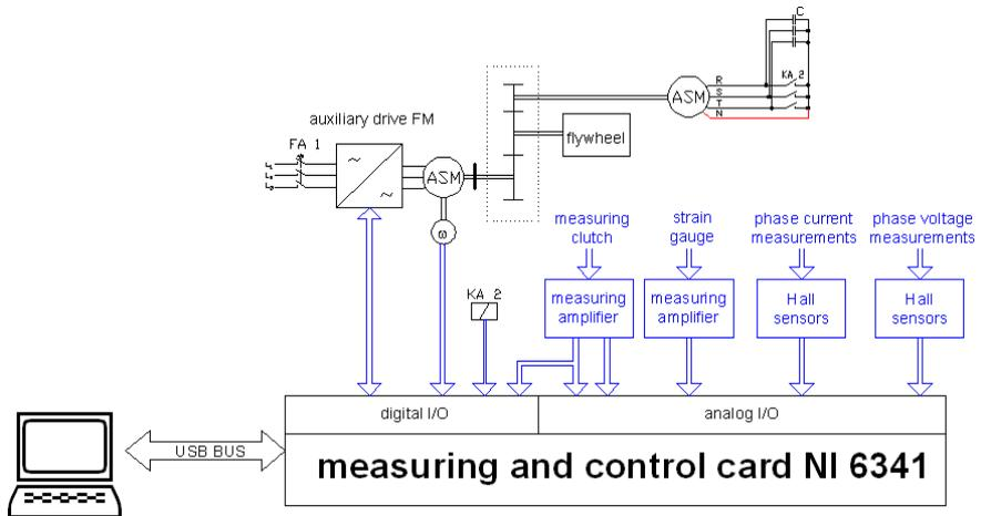
Fig. 2. The electrical structure of the laboratory test stand
