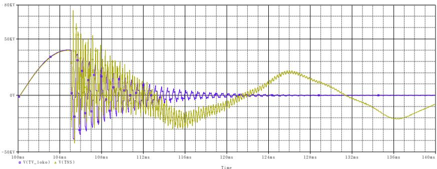
Fig. 2: The voltage waveform at FCD and recuperation mode of vehicle
