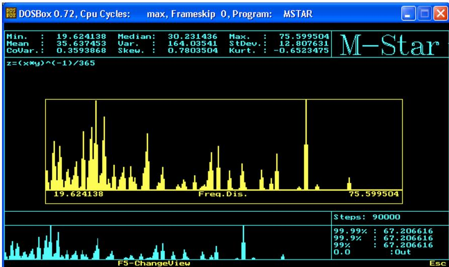
Fig. 16: Probabilistic lifetime calculation (temperature and dead weight influences) – MStar
