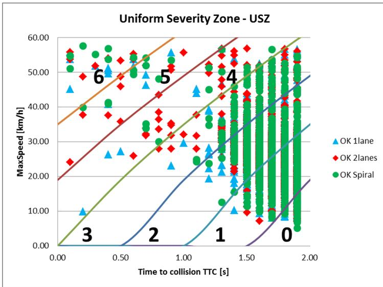
Fig. 8: Uniform severity zone for roundabout design alternatives
