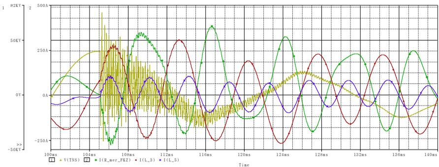
Fig. 3: The voltage and current waveform at FCD
