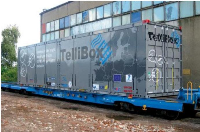
Fig. 3: TelliBox on low Sffgmrss type train [6]
