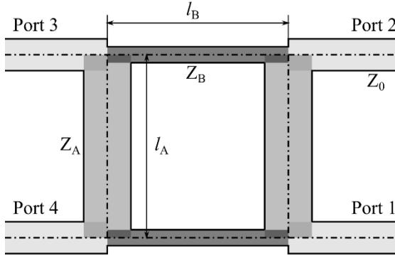
Fig. 5: One stage branch line divider circuit diagram
