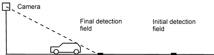
Fig. 9. Vehicle position after a change of the state of final detection field from “detection field occupied” to “detection field free”
