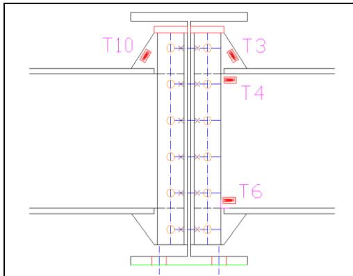
Fig. 12: Strain gauge positions
