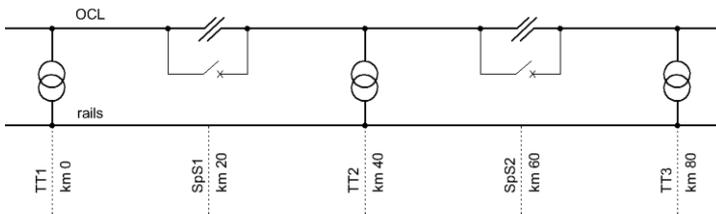
Fig. 3: Feeding diagram on AC system
