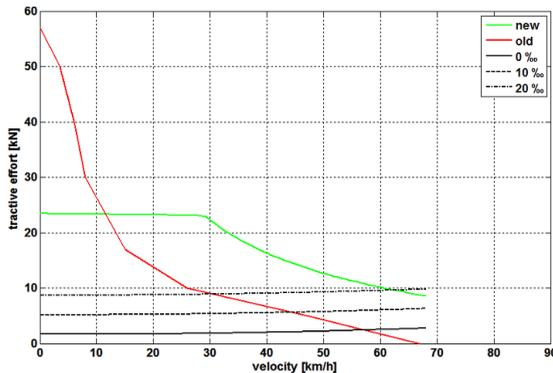
Fig. 5: Tractive effort curve of M27 after reconstruction (new) compared to tractive M27 before reconstruction (old)
