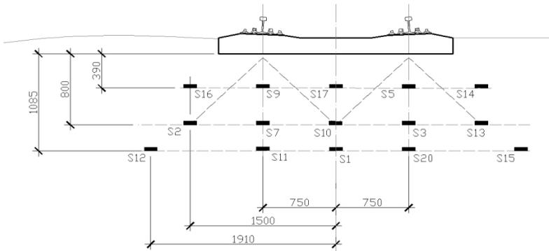
Fig. 1: Detailed description of pressure indicators placement
