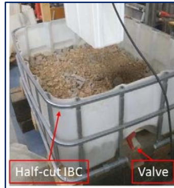
Fig. 2 Half-cut IBC with the drain valve
