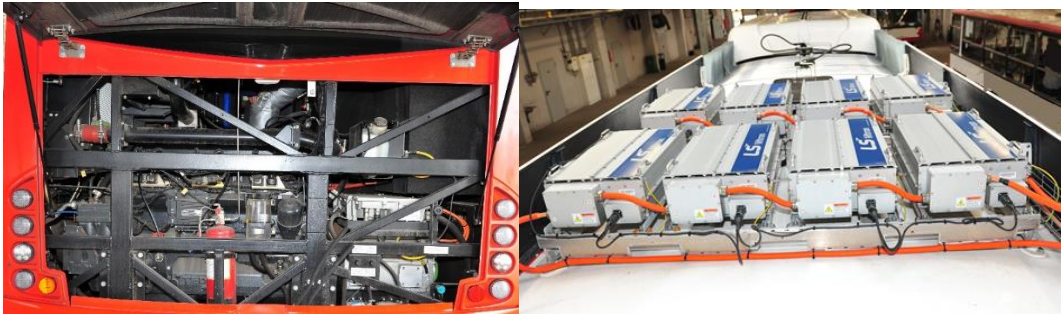
Fig. 1 Elements of a hybrid bus with drives: ZS-CNG-electric
