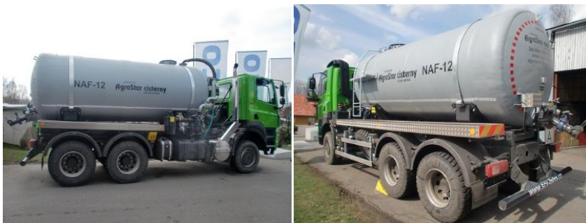
Fig. 1 Road tank anchored on the saddle supports [8]
