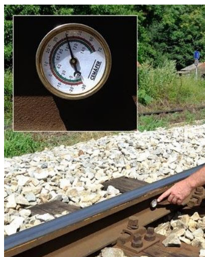
Fig. 6 Standard temperature measurement (Topčider measurement location in the vicinity of Belgrade, July 2017)
