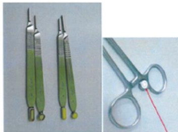
Fig. 3 Putting RFID chip into the separate case that is attached to the tool [18]
